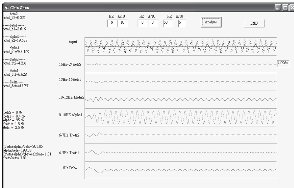
Fig. 5. Input 9 Hz with 60 Hz aliasing signals. The \alpha band there can be found to achieve 95%.
