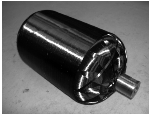
Fig. 5. Hoop winding (laminated continuously after helical winding).
