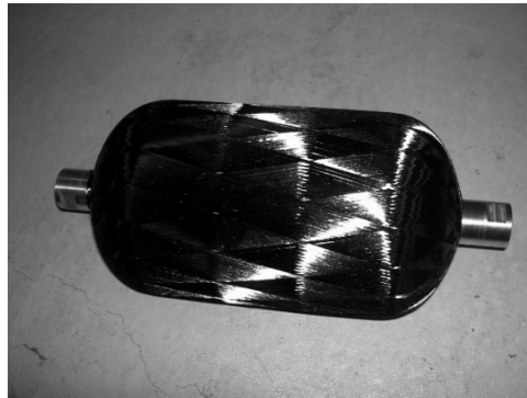
Fig. 4. Helical winding ( 16^\circ ).
