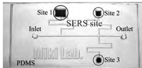
Fig. 8. Photograph of a manufactured microdevice containing silver nanoparticle sites and micro-channels.
