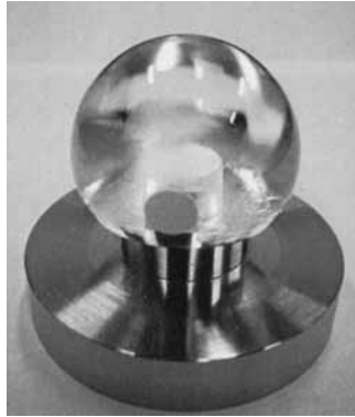
Fig. 2. Spherical single-crystal alpha-quartz specimen with Cr and Au films protecting the orientation-flat and bottom surface.
