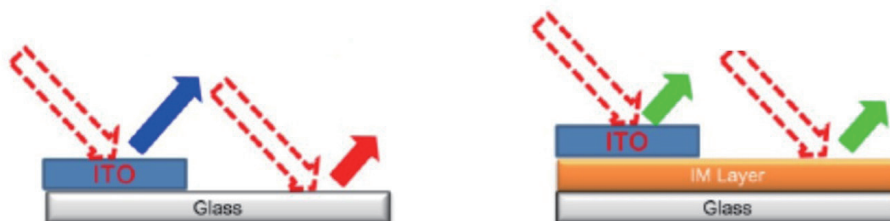
Fig. 4. (Color online) Design concept of the index-matching layer.
