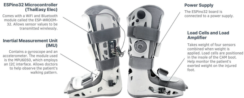
Fig. 2. Hardware: IoT gait pattern monitoring boots.
