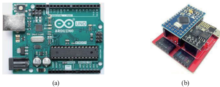
Fig. 1. (Color online) Arduino Uno and Webduino control panel. (a) Arduino Uno control panel. (b) Webduino control panel.
