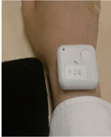
Fig. 1. (Color online) Loading position of three-axis accelerometer and gyroscope.
