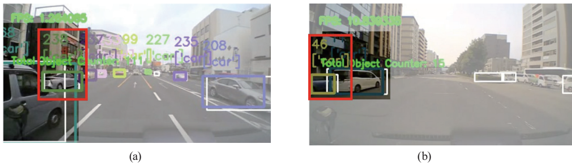
Fig. 10. (Color online) Two cases of on-street parked vehicle misclassified as moving vehicle.
