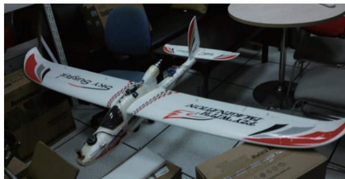
Fig. 2. (Color online) Fuselage after reinforcement and equipment installation.
