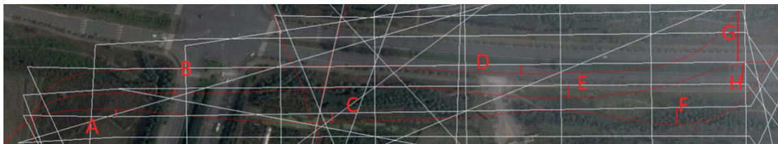
Fig. 7. (Color online) Flight tracks (red) and planned paths (white) in Experiment 1.
