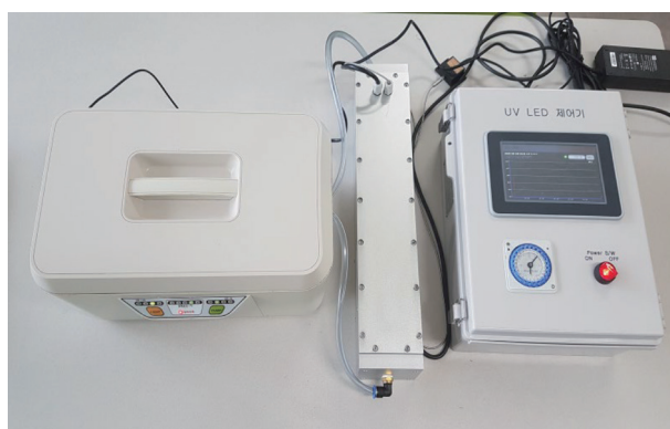
Fig. 6. (Color online) Experimental setup for UV-LED irradiation.
