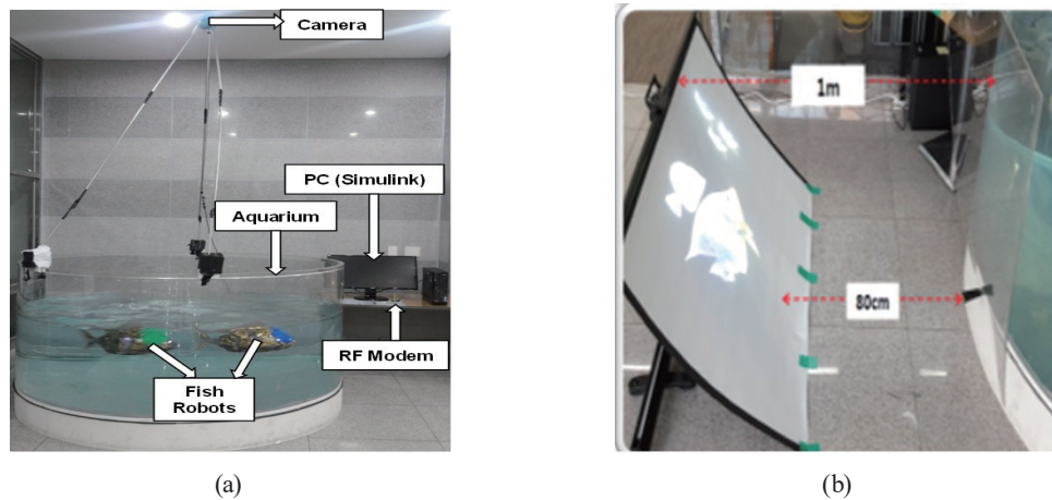
Fig. 5. (Color online) Experimental setup. (a) Monitoring of robot fish motion and (b) reflection of 3D hologram images by reflector.
