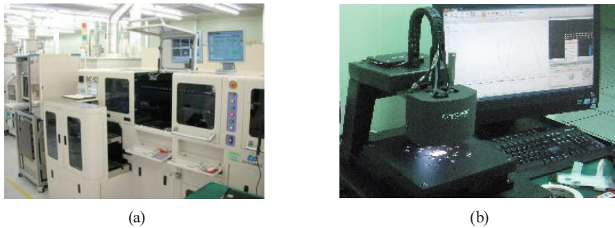
Fig. 14. (Color online) Experimental setups. (a) Laser drill machine. (b) Laser profile scanner.
