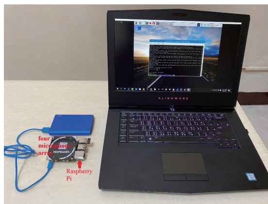
Fig. 4. (Color online) Experimental environment for Raspberry Pi and microphone array.
