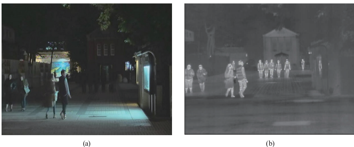
Fig. 1. (Color online) Comparison between images from (a) a visible camera and (b) a thermal camera.
