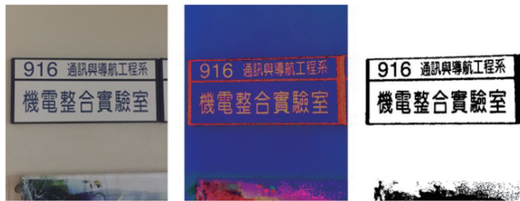
Fig. 5. (Color online) Doorplate images in RGB and HSV color spaces, and binary image.
