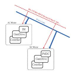
Fig. 2. (Color online) Structure of traditional heterogeneous motor drive system.
