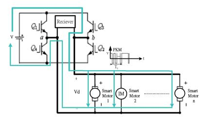
Fig. 7. (Color online) Communication signal transmission path of control command transmitted from front controller to smart motor.
