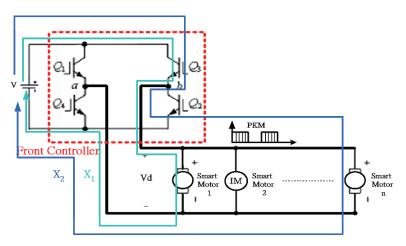
Fig. 10. (Color online) Current flow path in driving platforms for smart motors.
