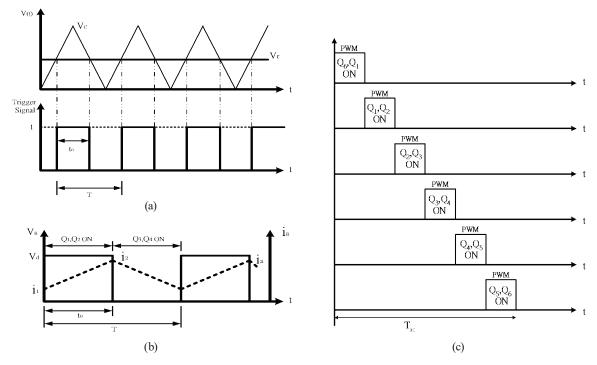
Fig. 4. PWM cycle operation. (a) PWM modulation method and waveform. (b) Current waveform during PWM period. (c) AC-motor drive strategy.
