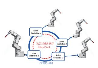
Fig. 1. (Color online) Robot arm drive architecture.
