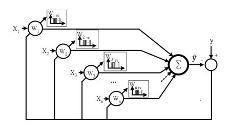
Fig. 9. Architecture of ADALINE artificial neural network.
