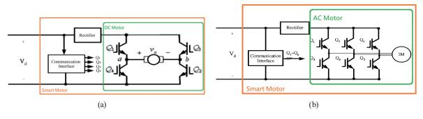
Fig. 3. (Color online) Architecture of smart motor. (a) Single-unit architecture of smart motor packaged with DC motor. (b) Single-unit architecture of smart motor packaged with three-phase induction motor.
