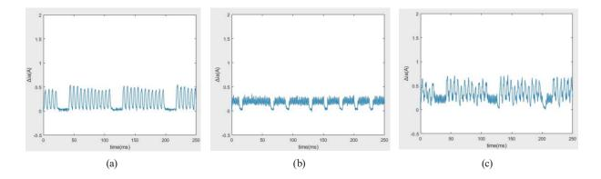
Fig. 25. (Color online) Current waveform sent back "01000011" to the front controller from both smart motor A and smart motor B by PKM strategy. (a)  $x_3 = \sin(2\pi \times 200)t$ , (b)  $x_{15} = \sin(2\pi \times 700)t$ , and (c) mixed waveform.
