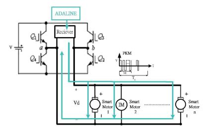
Fig. 12. (Color online) Communication signal transmission path of smart motor using ADALINE artificial neural network to send back information to front controllers.
