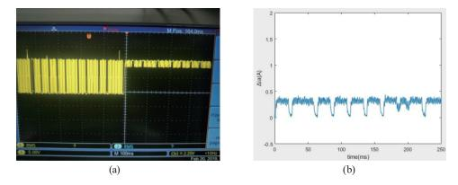
Fig. 23. (Color online) Front controller transfer command "00001010" and smart motor C carrier current waveform: (a) voltage waveforms during both  $T_t$  and  $T_r$  and (b) current returning waveform received by the front controller using current sensor.
