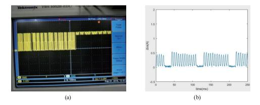
Fig. 24. (Color online) Front controller transfer command "00001010" and smart motor D carrier current waveform: (a) voltage waveforms during both  $T_t$  and  $T_r$  and (b) current returning waveform received by front controller using current sensor.
