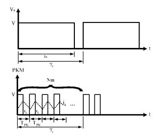
Fig. 11. Interior PKM technology driving strategy for smart motor in comparison with PWM technology.
