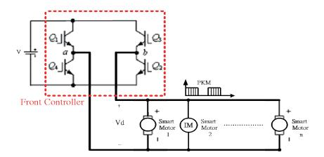
Fig. 5. (Color online) Architecture of smart motor drive system.
