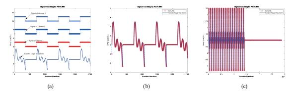
Fig. 22. (Color online) Simulation of three-channel communication for the ADALINE signal from the 1st, 3rd, and 5th channels. Transmitting and tracking results: (a) waveform before and after conversion, (b) results of overlaying convergence, and (c) transfer waveform.
