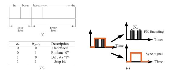
Fig. 6. (Color online) PK coding: (a) architecture of coding, (b) conversion table of data zone, and (c) wave form of coding.
