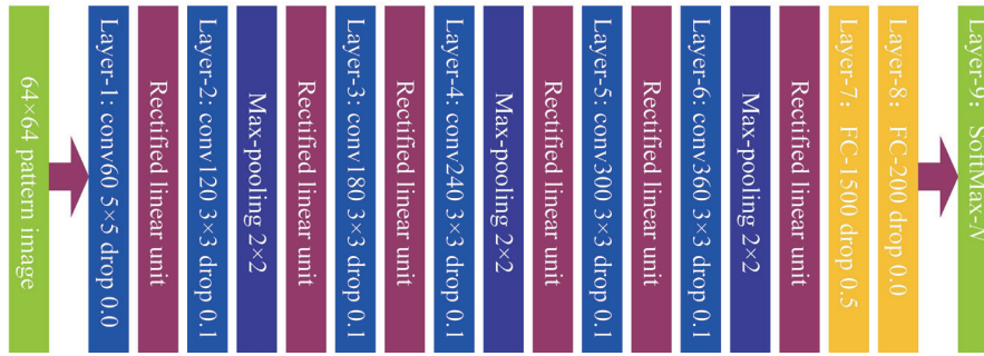
Fig. 4. (Color online) Architecture of deep convNet for convNet-based feature extraction.
