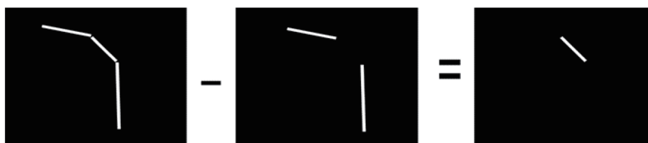
Fig. 11. Subtracting a background image obstructed by a solid object from a clear background image yields a complete image of the object.
