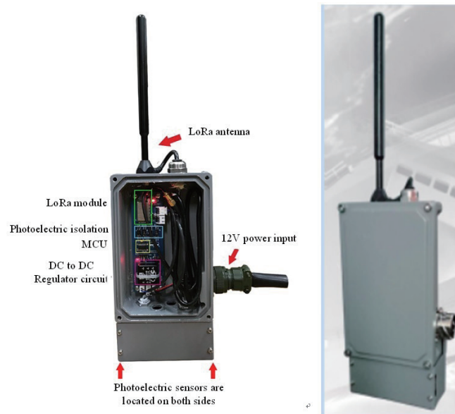
Fig. 16. (Color online) Infrared electric fence circuit combined with aluminum 6061 housing.
