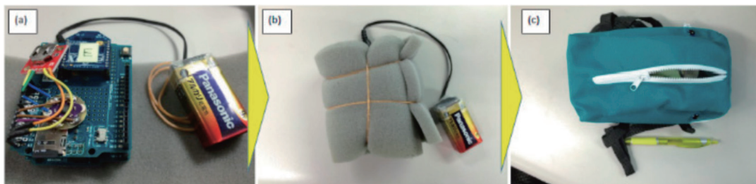
Fig. 4. (Color online) (a) Animal-to-animal data sharing prototype, (b) covered by sponge for protection from shocks, and (c) placed in the bag. (7)
