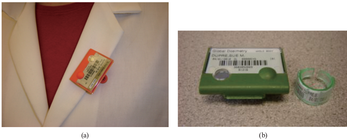
Fig. 12. (Color online) (a) Nametag on the badge is oriented in the opposite direction from the body and (b) radiation film badge. (16)
