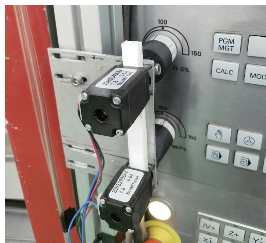
Fig. 3. (Color online) The knob adjustment mechanism is composed of stepper motors and plastic sockets. The upper knob is the spindle speed knob and the lower one is the feed rate knob.
