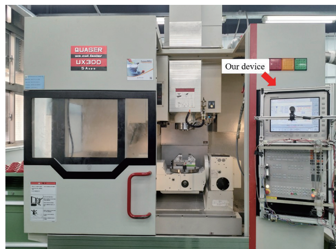
Fig. 4. (Color online) The add-on device was installed on the control panel of the CNC machining center.
