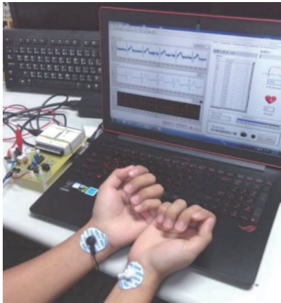
Fig. 6. (Color online) ECG signal capturing circuit.
