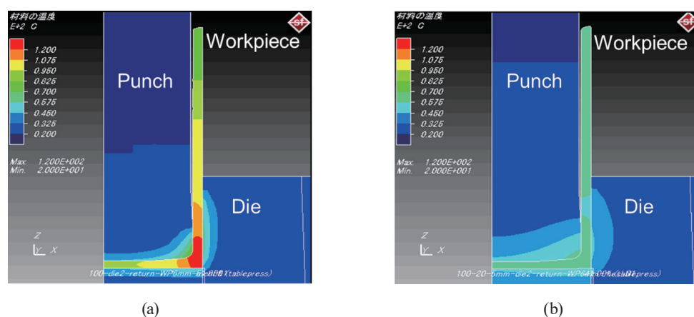
Fig. 6. (Color online) Temperature distribution with different punch speeds in forging process. (12) (a) Punch speed: 100%. (b) Punch speed: 100% → 20%.
