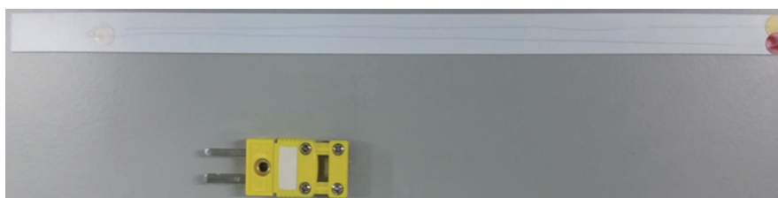
Fig. 2. (Color online) Bare-wire-type thermocouple (top) and thermocouple connector (bottom).
