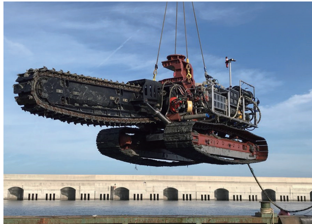
Fig. 1. (Color online) Track-based underwater construction robot under development.
