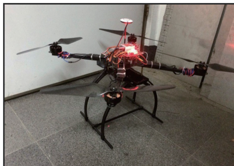
Fig. 11. (Color online) Quadrotor installed with a smartphone camera.
