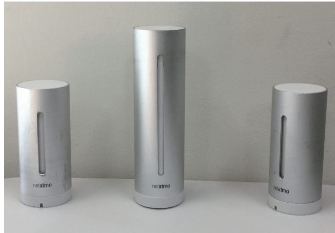
Fig. 2. (Color online) Netatmo sensors used: (left to right) outdoor module, indoor module (base station), and indoor module (additional module).
