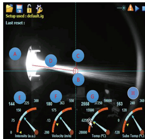
Fig. 3. (Color online) Real-time monitoring system for spray flame flow.
