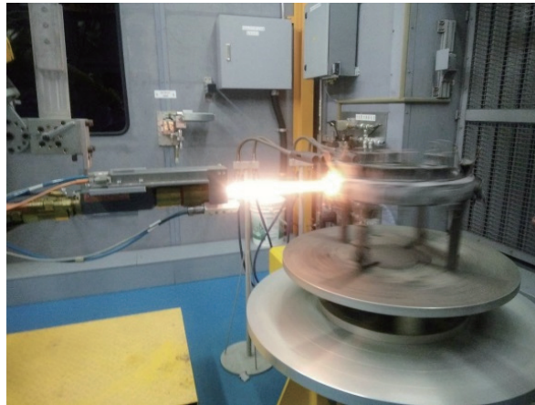
Fig. 2. (Color online) Test piece being sprayed using HVOGF or HVOLF.
