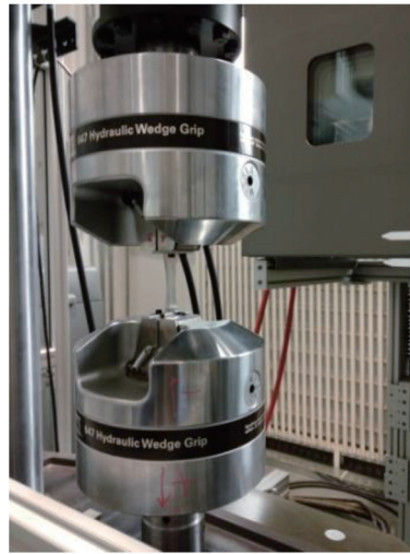
Fig. 7. (Color online) Installation of fatigue test specimens.
