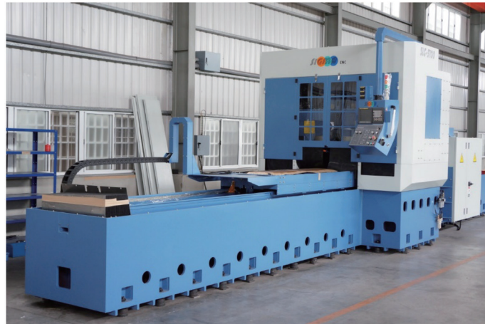
Fig. 1. (Color online) Target three-head grinding machine.
