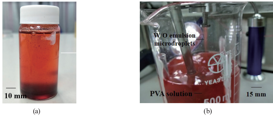
Fig. 6. (Color online) (a) View of DOX mixed with 5% w/w PCL solution. (b) View of W/O emulsion microdroplets obtained using the atomizer.
