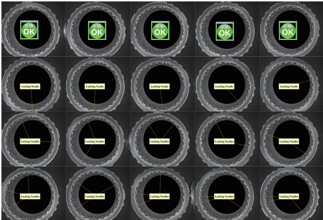
Fig. 16. (Color online) Online inspection results of qualified and defective parts.
