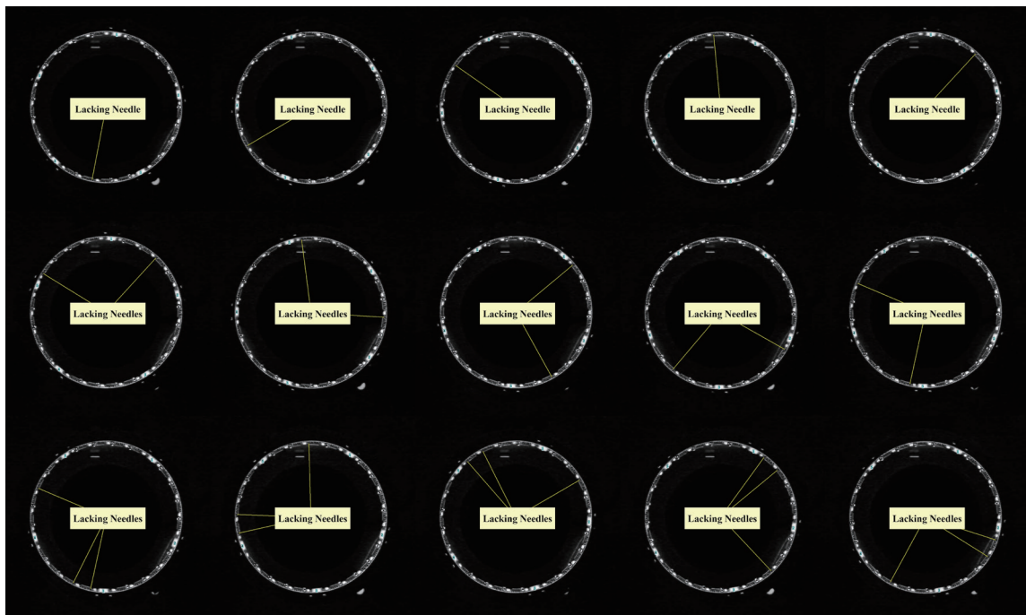
Fig. 12. (Color online) Offline inspection results of lacking needles.
