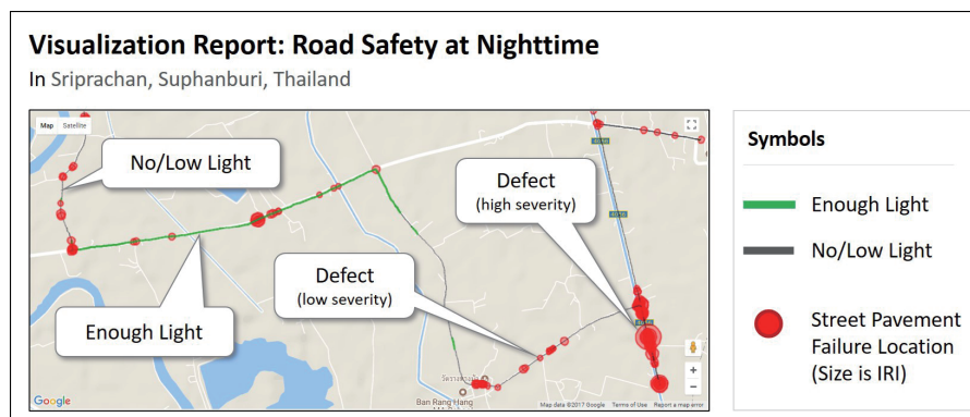
Fig. 9. (Color online) Visualization report for monitoring roadway lighting and pavement defects at nighttime.
