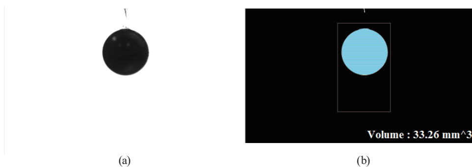
Fig. 5. (Color online) Volume calibration of the bearing ball of 2 mm diameter: (a) a picture of the bearing ball and (b) an image contour of the bearing ball picture with the volume presented.
