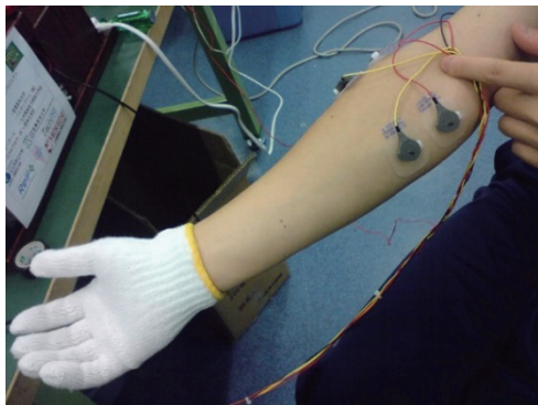
Fig. 3. (Color online) Positioning of myoelectric sensors.
