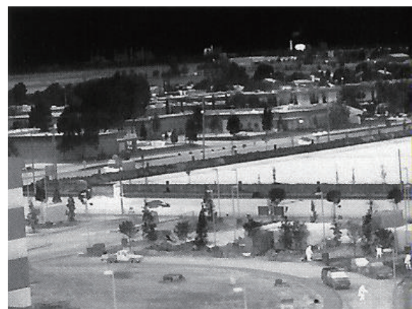
Fig. 8. Example of thermal image taken with IR-M700 using 801 \times 512 PtSi SB IRFPA.
