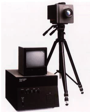
Fig. 7. (Color online) First commercial staring infrared camera IR-5120A with 512 \times 512 PtSi SB IRFPA.
