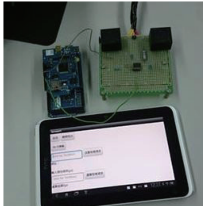
Fig. 15. (Color online) Setup for the remote power signal measurement implementation.
