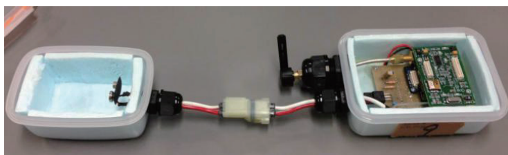
Fig. 2. (Color online) Power supply system upgraded wireless acceleration sensor.
