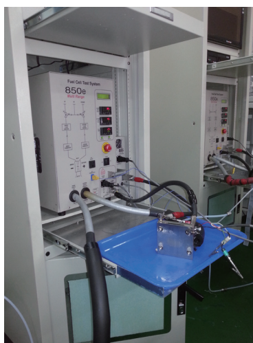
Fig. 6. (Color online) Fuel cell test system used in this work.
