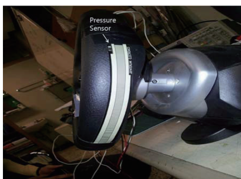
Fig. 9 (left). (Color online) Gripping force pressure sensor attached to steering wheel. Fig. 10 (right). (Color online) Gripping force sensor circuit.
