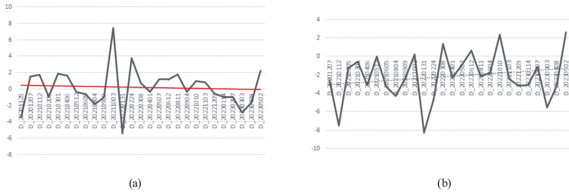
Fig. 17. (Color online) PS-InSAR and SBAS-InSAR results. (a) Folded graph of the change in settlement at a PS point. (b) Folded graph of the change in settlement at a point of SBAS.
