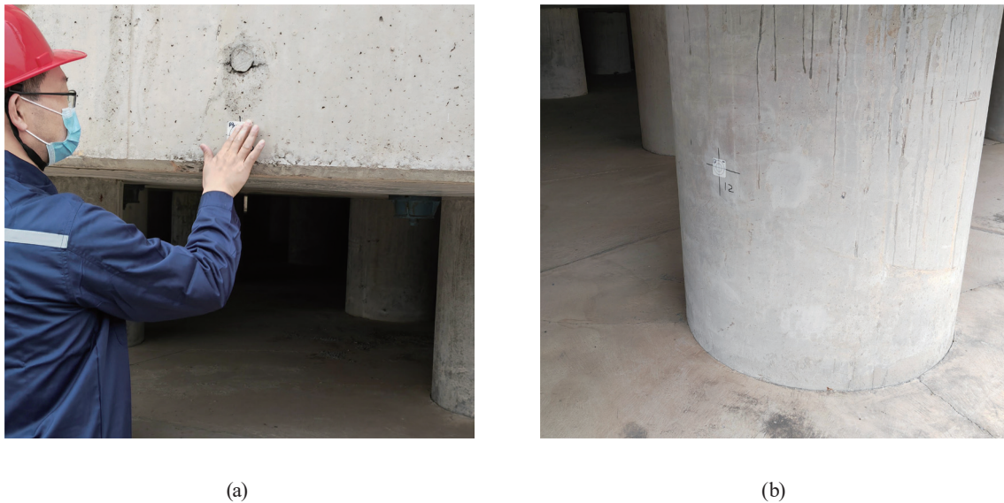
Fig. 4. (Color online) Attaching reflective sheet. (a) Site of attaching reflective sheet. (b) No. 12 reflector location.
