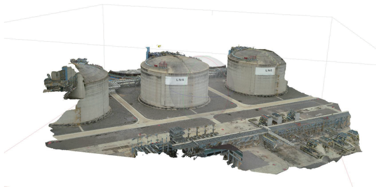
Fig. 9. (Color online) Oblique photography to generate point cloud data.
