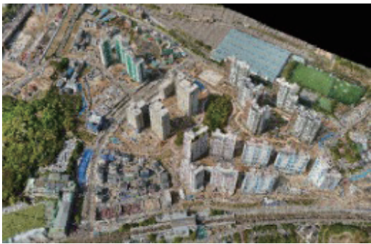
Fig. 2. (Color online) Generation of 3D high-density point cloud data.
