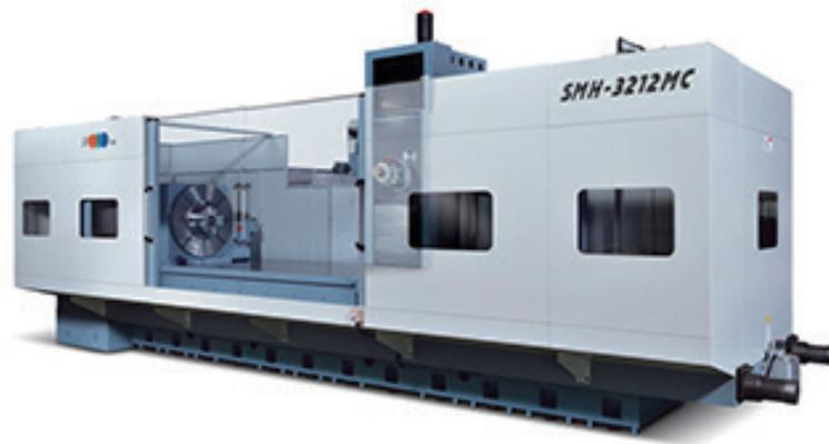
Fig. 13. (Color online) Final HMC optimized via the proposed design methodology.
