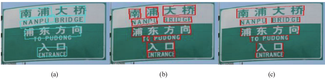
Fig. 8. (Color online) Comparison of detection by models under conditions with dense text: (a) EAST, (b) Advanced EAST+VGG16 256, and (c) Resnet50+Advanced EAST Fixed Size 256.
