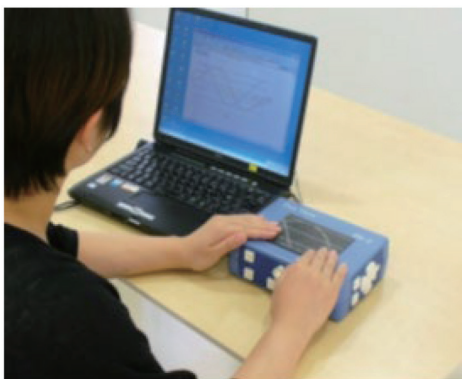
Fig. 1. (Color online) Braille graphic display.
