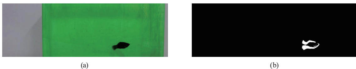
Fig. 15. (Color online) Example of failures in the extraction of the fish region. (a) Target frame. (b) Fish region extracted from (a).
