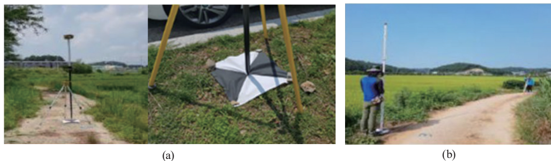
Fig. 4. (Color online) Photographs of (a) horizontal GNSS Network-RTK survey and (b) vertical level survey.
