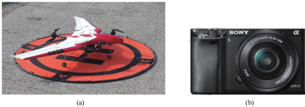
Fig. 5. (Color online) Photographs of (a) FireFly6 Pro and (b) Sony a6000 camera.
