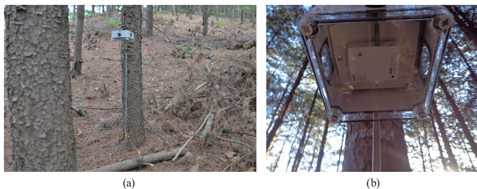
Fig 2. (Color online) HOBO data logger installed at site 6 (PK forest stand) as the instrument ( 15 \times 15 cm 2 , height 1 m) for measuring micro-meteorological factors.
