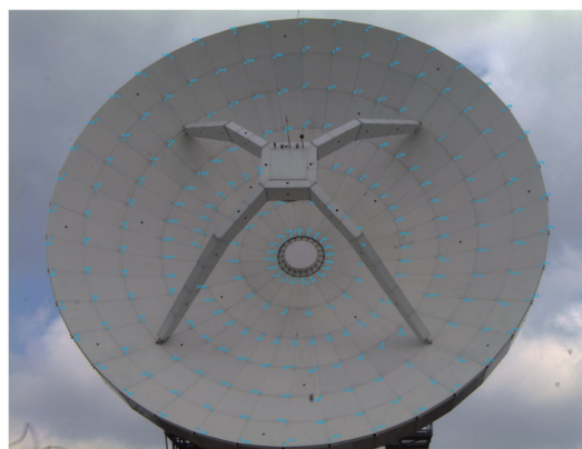
Fig. 2. (Color online) Feature points distributed on the inner surface of the parabolic reflector labeled to match the measurement results of image and control point coordinates.
